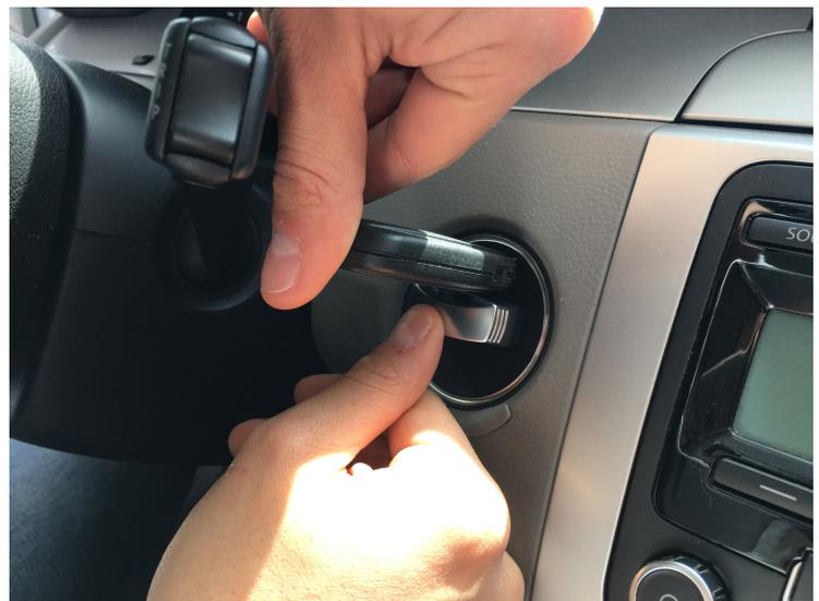
6. The software will prompt you to insert the TA31 extractor into the PROTAG programmer once it is ready and will display you the PIN code. This will allow you to program a spare key to the car.
