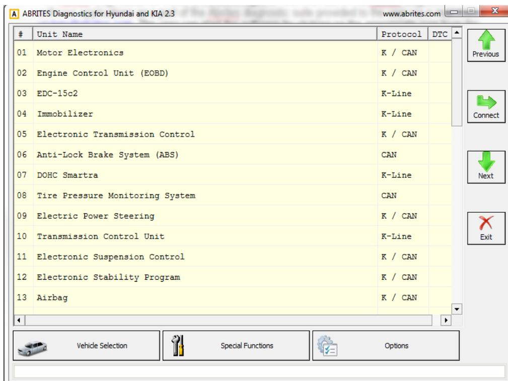
This is the main diagnostic screen of the software. It contains the navigation buttons and provides a list of all the electronic modules that March be integrated into Hyundai and Kia vehicles.
