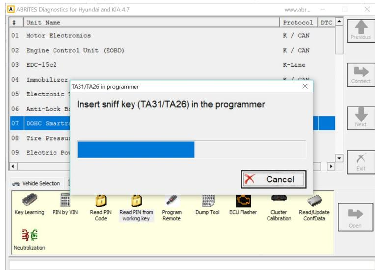
4. Remove the working key and switch the IGN ON 3 times together with the working key and TA31:
