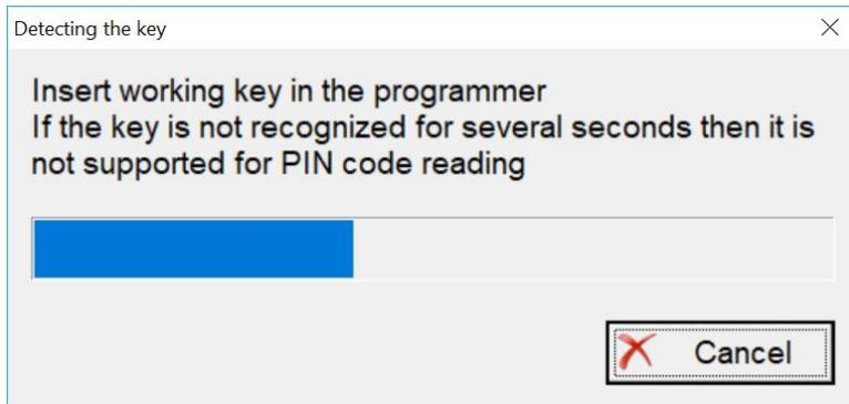
3. Remove the TA31 extractor when prompted and insert the working key into the PROTAG programmer
