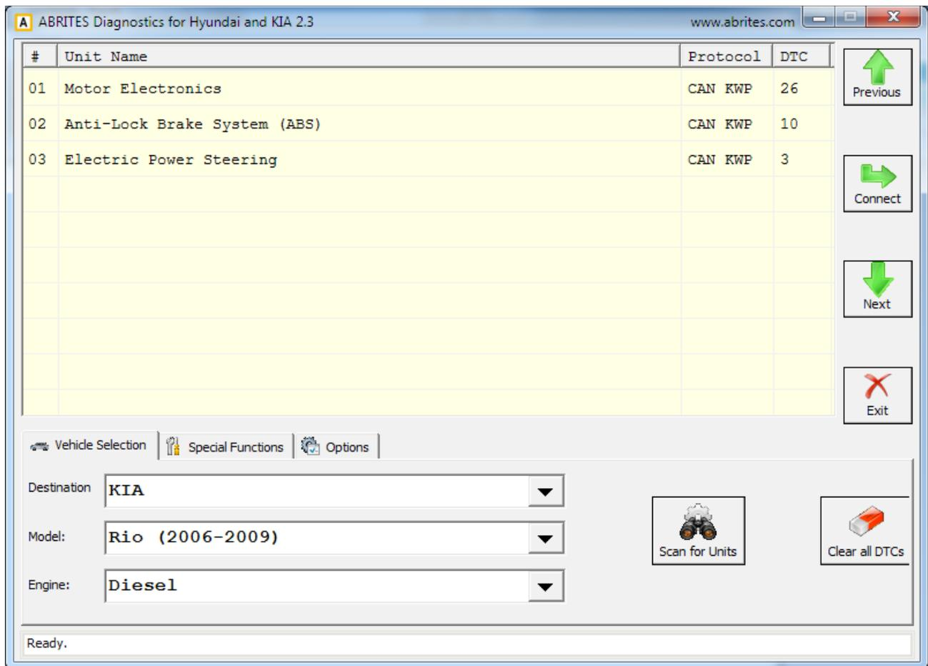
Once the vehicle is selected the Abrites diagnostics for Hyundai and Kia will display all the possible modules that may be integrated into this specific vehicle. It will display all the protocols in which these electronic components communicate.
