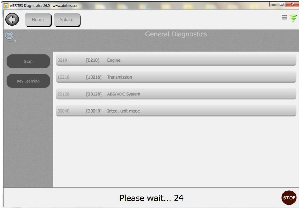
Once the scan is complete the user can enter an electronic module by clicking on it.
