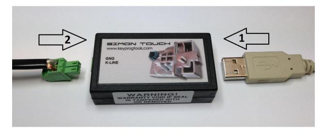
8 - Connect the MBSTEERING ground to the ESL ground Connect the MBSTEERING K Line to the ESL K Line
