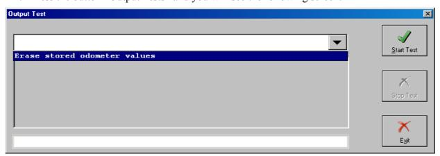
Select "Erase stored odometer values" and press the button "Start". Wait 1 second and then close the screen.
