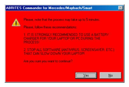
You should pay attention to this warning and make sure your laptop is powered with a constant power supply. The process takes less than 5 minutes, so usually it is not necessary to use a booster for the battery of the car.
