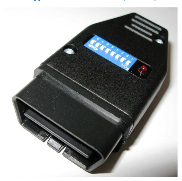
Device can perform bypass of the immobilizer of the vehicles equipped with engine control units from BOSCH:
