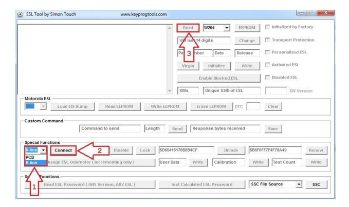
• Device will read the SSID/Hashes ESL Status, Motor position and show you ESL IS NOT REPARABLE.
