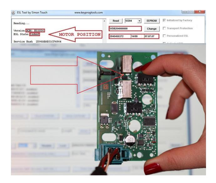
• Press and hold the 2 switches and click on read. Software will show the ESL in Unlocked position.
